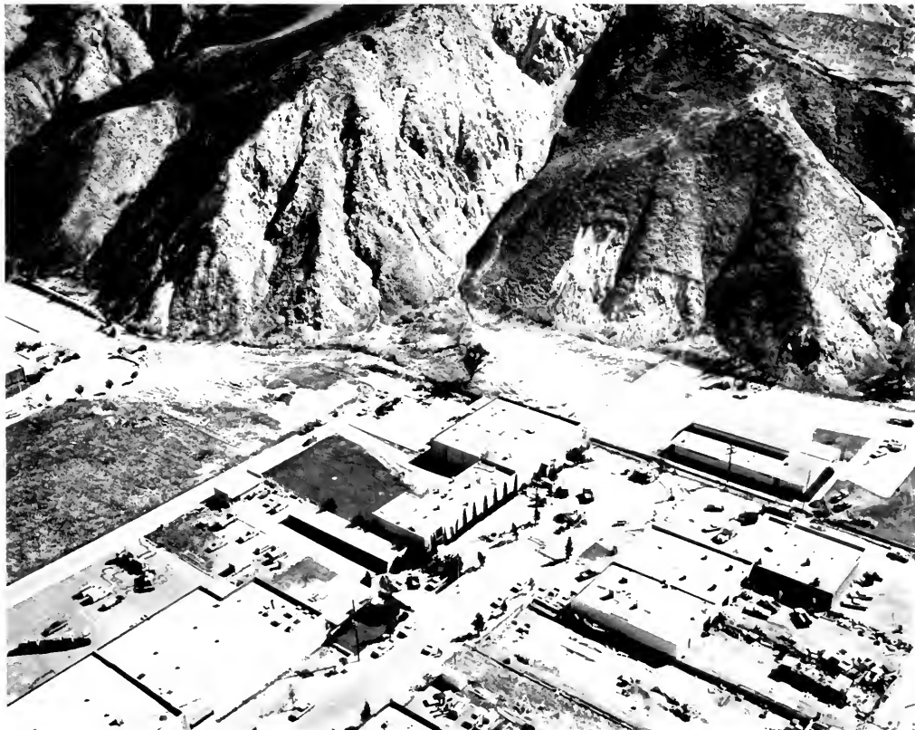
Photo 1. Abundant shallow small slope failures in Towsley and Madelo Formations near San Fernando Ranger Station. Photo courtesy of Los Angeles Department of Building and Safety.
